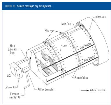
entering the cabin during take-off and ascent while the envelope air is still warm. It could also be used for venting the envelope while the plane is on the ground, with a hot air supply for example.
