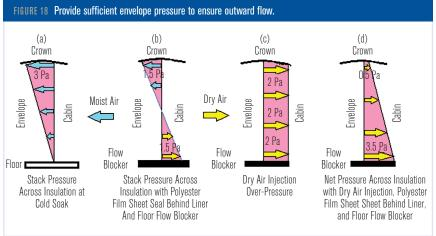
smaller amount of dry injection air required, perhaps no more than one-tenth of the amount of current CCDS dehumidified airflow rates. Just inserting a flow blocker at the floor could reduce condensation rates by as much as 50% (*Figure 18b*). The 0.5 Pa (0.002 in. w.g.) minimum net pressurization of the envelope relative to the cabin is chosen to minimize any molecular back diffusion of cabin water vapor into the envelope through small leakage openings.
