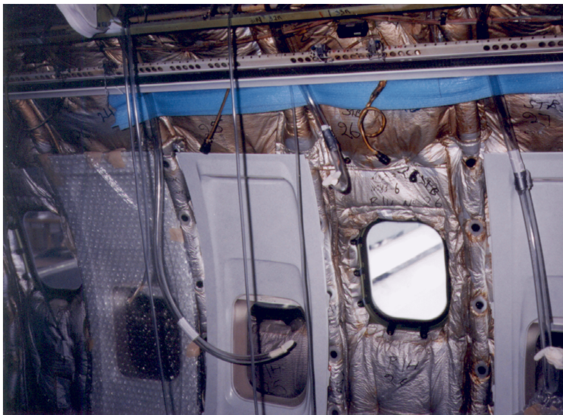
Figure B.5 View of the B737 Sections 24, 25 and 26 (port side) injection air tubes, pressure and VOC sampling tubes, and Section 22 pressure sampling tubes with the cabin stowage bins removed
