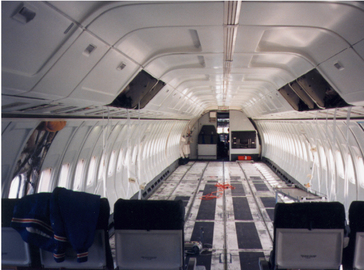
Figure B.1 View of the B737 cabin interior showing port and starboard cabin envelope sensor tubing
