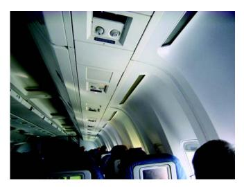
Figure 1 Economy section in a wide-body passenger aircraft cabin showing several overhead personal service units with their individually controlled gaspers (personal air outlets) and reading lights. The main cabin ventilation supply is provided by sidewall slot diffusers located just below the overhead stowage bins and ceiling slot diffusers located just above the stowage bins near the aisle. IAT photo May 14, 2010.
